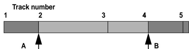
If the A point is set at the start of a track, and the B point at the end of another track, the whole of the tracks containing and between these points will be erased (in the example above, tracks 2 and 3 will be erased).
